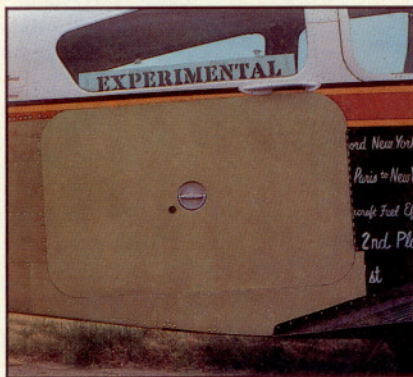
An enlarged cargo door, such as this one, or the standard cargo door may be ordered as part of the Tri-Tail conversion.
