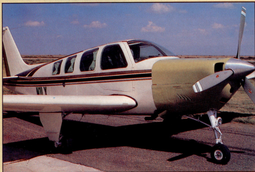
A new aluminum and fiberglass cowling has been designed to house the 400-hp engine.
